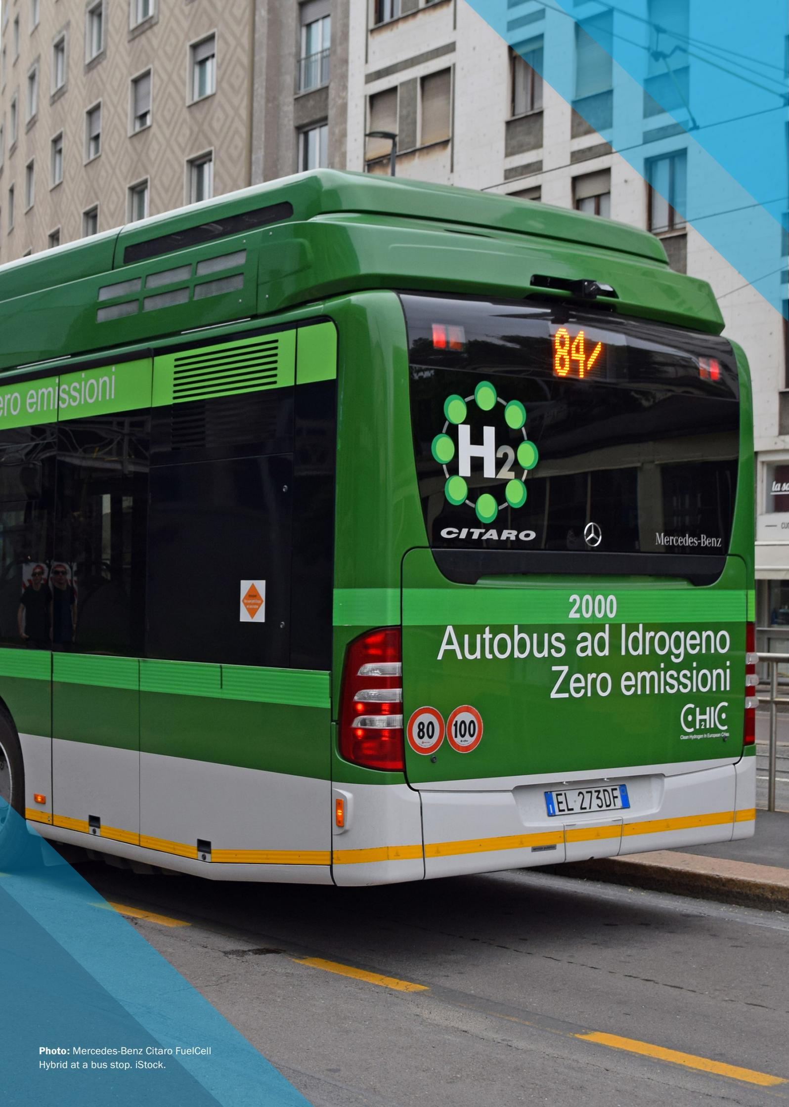
Photo: Mercedes-Benz Citaro FuelCell Hybrid at a bus stop. iStock.
