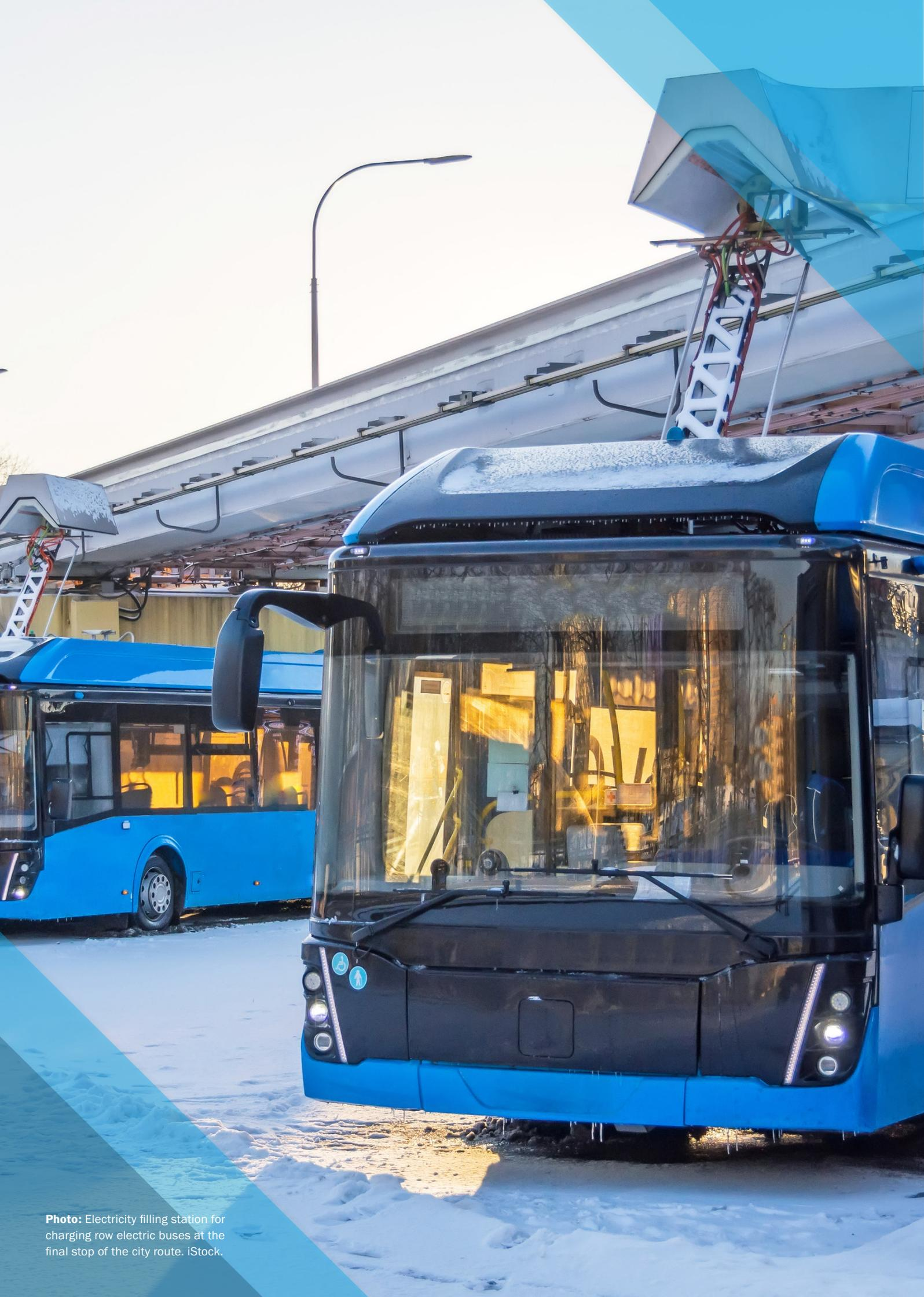
**Photo:** Electricity filling station for charging row electric buses at the final stop of the city route. iStock.
