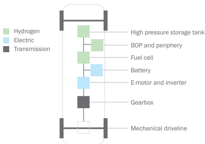
The fuel cell acts as the onboard electric energy source, generating electricity both charging a small battery and powering the electric drive.
