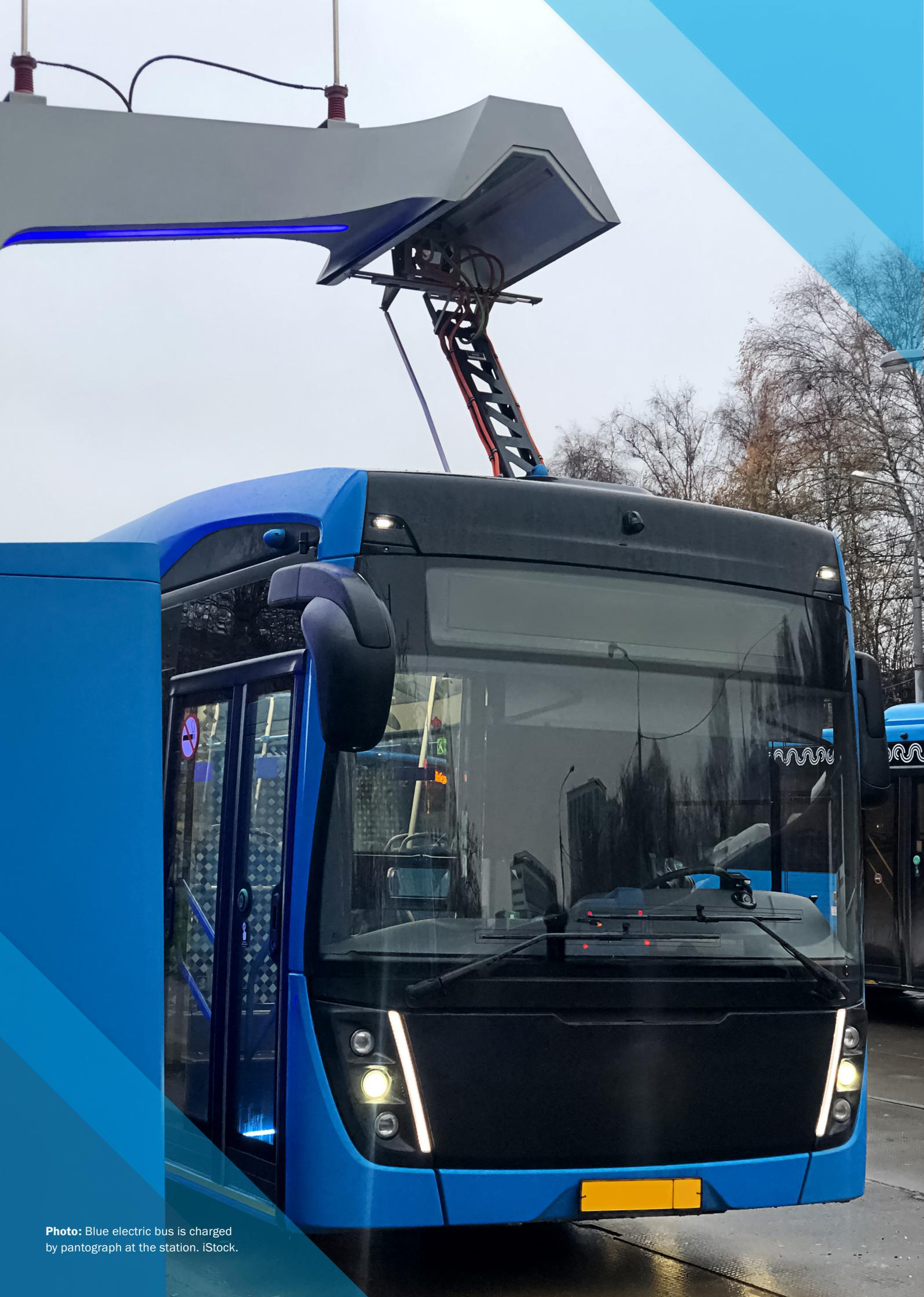
**Photo:** Blue electric bus is charged by pantograph at the station. iStock.
