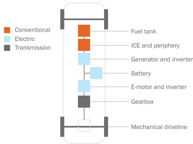
In other words, the hybrid technology combines the best aspects of both conventional and electric technologies: the high energy density of conventional fuels with the high efficiency of the electric powertrain to generate work. Therefore, hybrid buses present driving ranges in excess to those of conventional buses, which combined with short refueling times result in high operational flexibility.<sup>22</sup>
