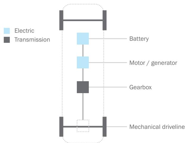
The vehicle consists mainly of a battery where electric energy is stored, an electric motor/generator, and the transmission.
