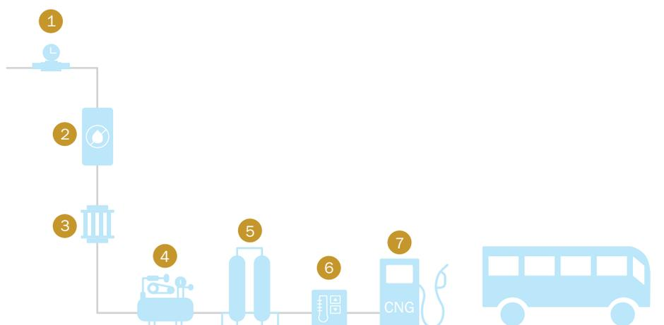
1. **Gas line:** the gas line serves as the fuel input to the CNG refueling station. The gas is delivered directly to the station through the regional gas distribution grid. The gas line is connected to the grid through a utility gas meter which measures the overall gas consumption of the whole station.
